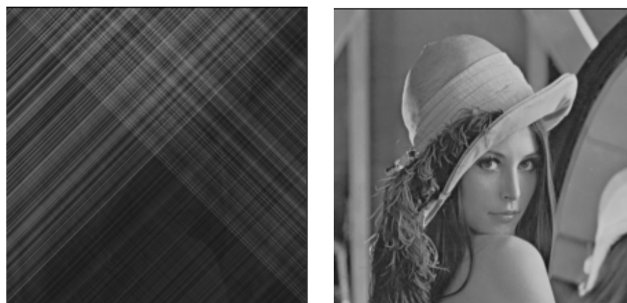
Figure 14. Encrypted grayscale images and restored images in the proposed method of this study. The figure on the left is the encrypted grayscale image; the figure on the right is the restored image.
